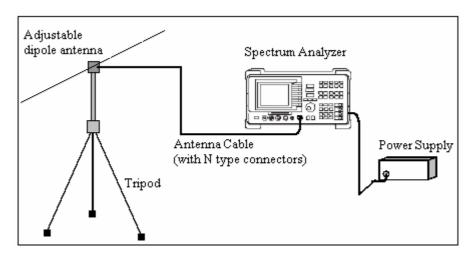
Figure 1: Measurement set-up
