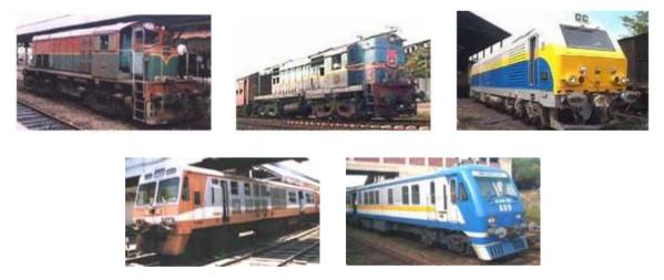
Figure 2: M7, M8 and M9 Diesel Locomotives (top) S8 and S9 DMU Locomotives (bottom) [11]
