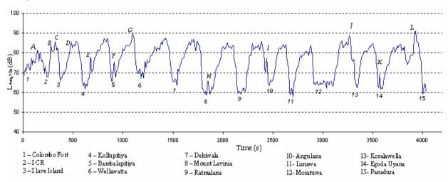
**Figure 3**: Noise levels for a M9 Diesel locomotive traveling from Colombo to Panadura. Minima in the figure correspond to the location of the stations.
