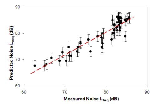
**Figure 8**: Measured and predicted noise levels for the acceleration phase. The three symbols represent three different sections of the journey. The error bars indicate the 2.0 dB uncertainty in the predicted values.
