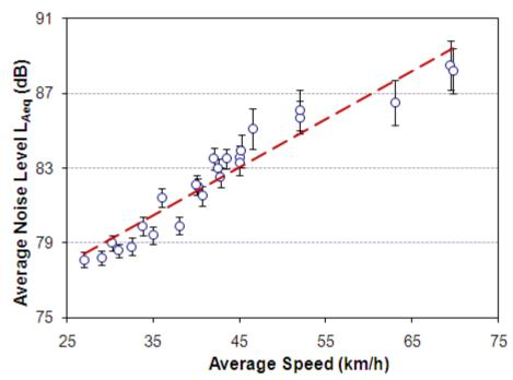
Figure 5: The average noise level within rail compartments as a function of train speed
