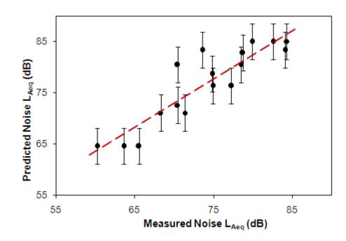
**Figure 10:** Measured and predicted noise levels for the deceleration phase. The three symbols represent three different sections of the journey. The error bars indicate the 3.5 dB uncertainty in the predicted values.
