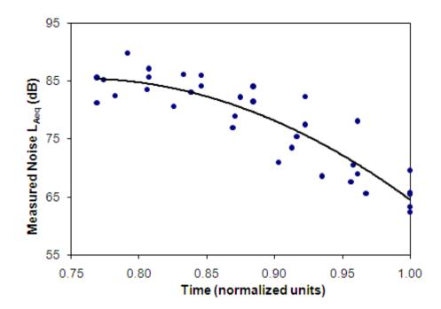
Figure 9: Average noise levels during the deceleration phase as a function of time
