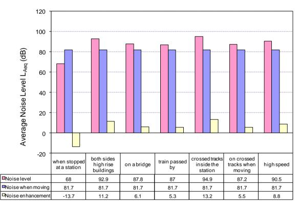
Figure 4: Noise enhancement due to external parameters
