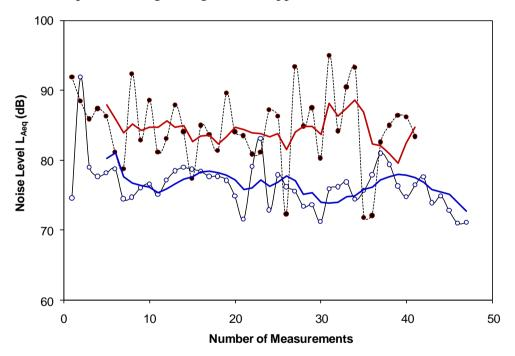
**Figure 6**: Comparing the noise level in the guardroom with the noise level in the 5<sup>th</sup> passenger compartment of a M9 locomotive running at an average speed of 35 km/h.
