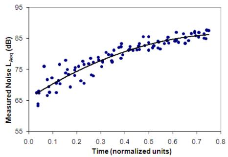
Figure 7: Noise levels during the acceleration phase as a function of time
