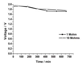
Figure 4: Discharge curves for the cells, Mg / GPE / C:  $I_2$  under constant loads of 1 M $\Omega$  and 10 M $\Omega$  at 28°C
