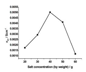
Figure 1: Room temperature conductivity variation with Pr<sub>4</sub>NI concentration (by weight)
