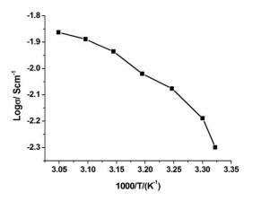
Figure 2: Temperature dependence of the conductivity of the sample which showed the highest conductivity at 28°C
