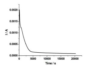
Figure 3: DC polarization curve taken with blocking electrodes at 28°C
